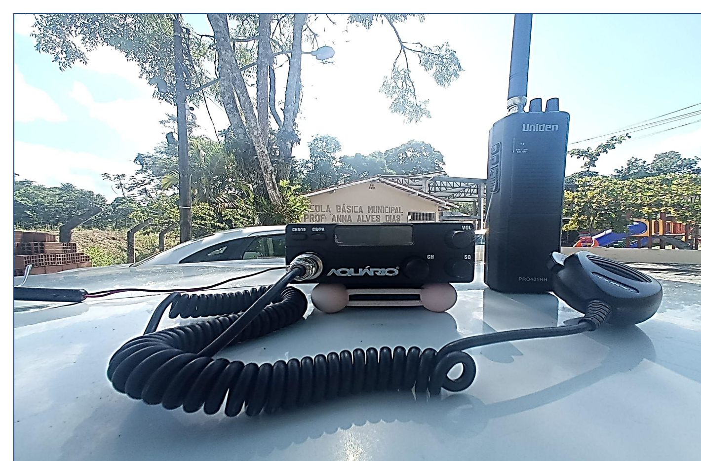
Figure 02: Equipment used in the reception test. Aquarius RP40 and Uniden PRO401HH (The authors)
